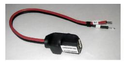
The WiFi Power Cable uses the Online Controller's ModBus power and puts it into a USB female connector. However, the voltage supplied by the ModBus power is significantly higher than the USB standard allows (12V vs. 5V)! The listed wireless access points are able to work with this higher voltage, however, if using a different access point, check first with it's power supply specifications.
